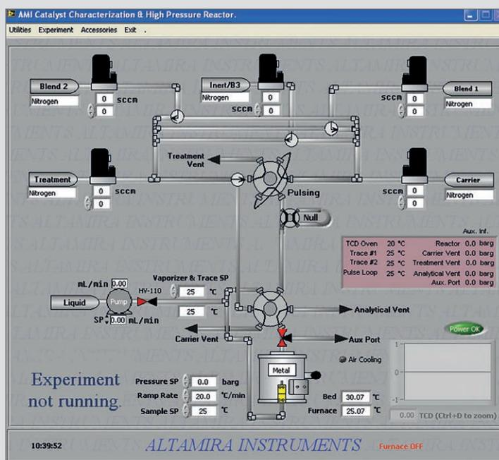
Figure 12 Operating Screen - A complete overview of all experimental parameters
