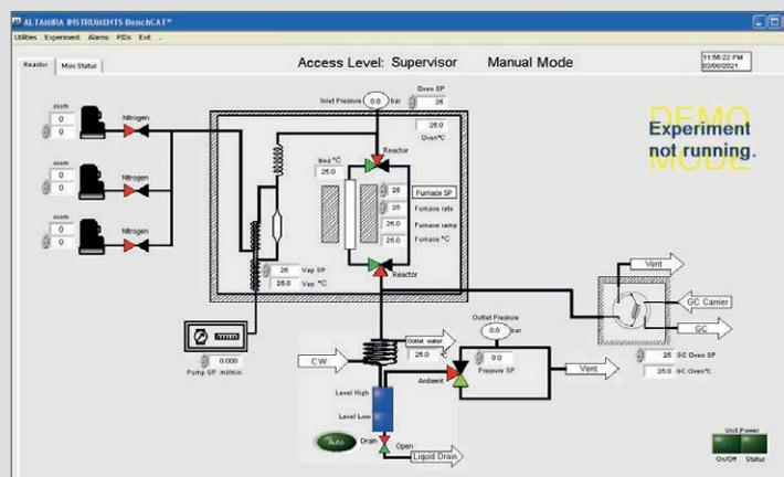
Figure 16 Main Operation Screen of the μBenchCAT
