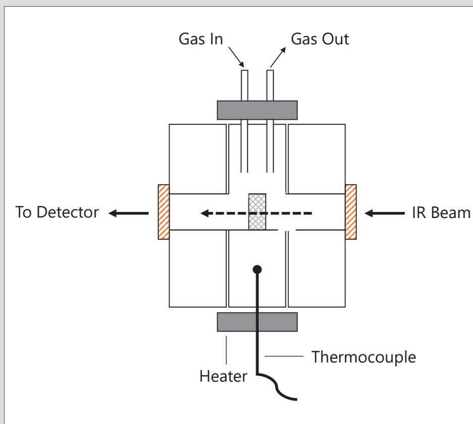
**Figure 3** Diagram of IR transmission cell
