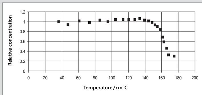
**Figure 7** Isobar of CO adsorbed on 1% Pt/Al<sub>2</sub>O<sub>3</sub>
