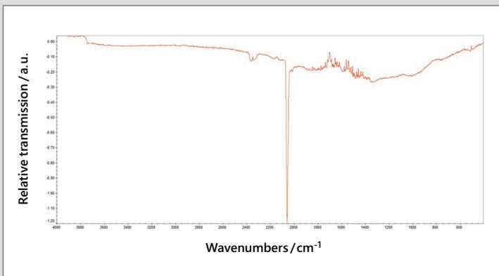
**Figure 5** IR spectrum of CO adsorbed on a 1% Pt/Al<sub>2</sub>O<sub>3</sub>.
