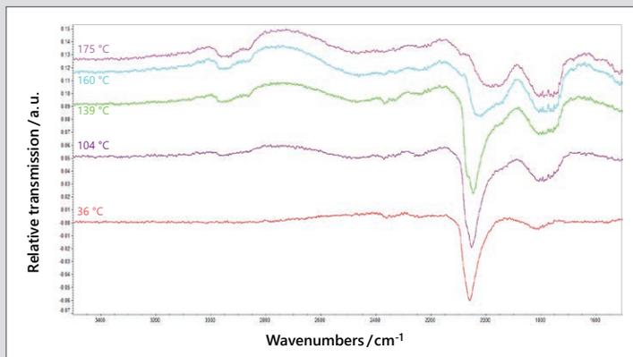
**Figure 6** CO signal as a function of temperature
