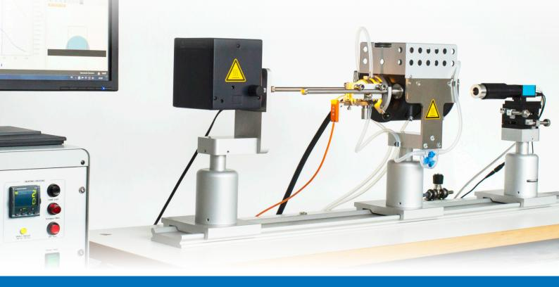
Determine the characteristic temperatures according to international standards of ash fusibility
