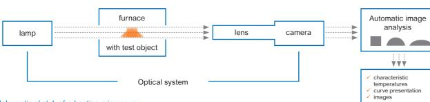
Schematic sketch of a heating microscope
