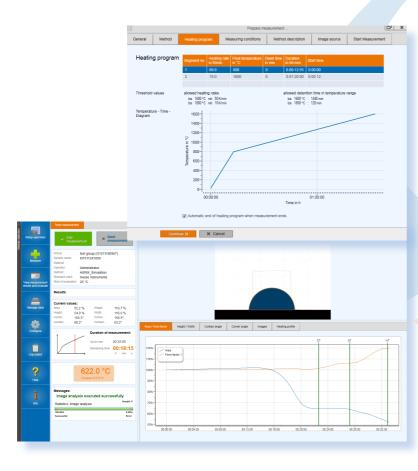
Evaluation: When a measurement has been completed, the results page is displayed with the measurement values, characteristic temperatures, graphical presentation of the results and images. A standardized one-sided summary record can be used as a clear test report. All of the important measurement conditions and results and images of test object silhouettes are documented and a comment in text form can be added.
